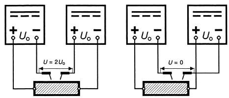
Figure A: Example of d.c. voltage between electrode holders or torches
